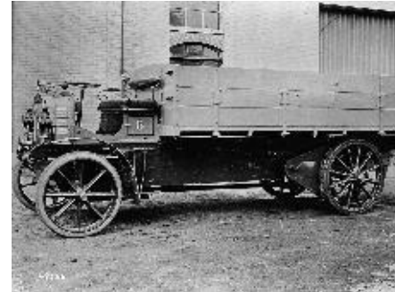
As of 1900 GF develops wheels made of cast steel for trucks and cars
